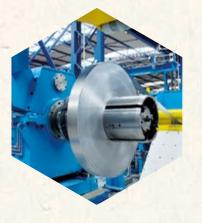
In the years 2002-2008, Ferona Group's network of cutting centres was gradually built, focusing on the transverse and longitudinal cutting of coil sheets. According to the needs of Ferona's customers. these Steel Service Centers in Hradec Králové, Ostrava and Bratislava process more than 300,000 tons per year of both cold-rolled and hot-rolled material.
